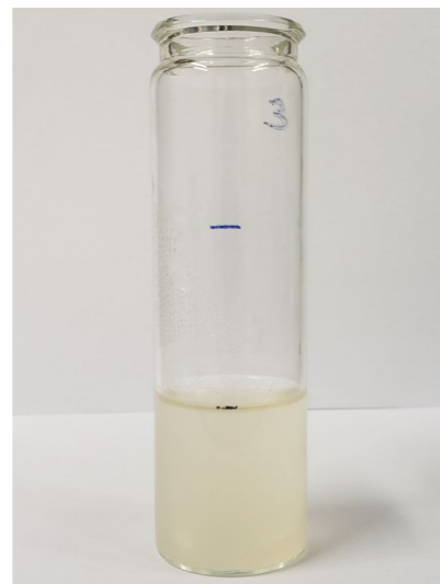
Fig. 1. Example of a container filled with clear gelatin after Step 1e. This example shows the level of clarity needed to see diffusion readily. Even clearer gelatin just makes measurements easier.
